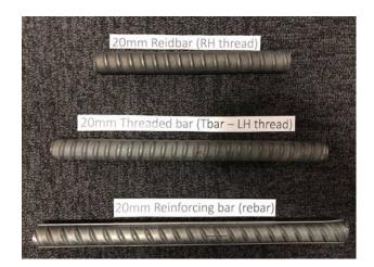
The imported goods, whether they be reinforcing bar or threaded bar will have a range of different rib patterns as this aspect is not defined by a Standard, rather the proportion of the bar surface requiring deformations to be present. The Standard to which the imported threaded bar, and domestic rebar is being produced, namely AS/NZS 4671:2001 states:
