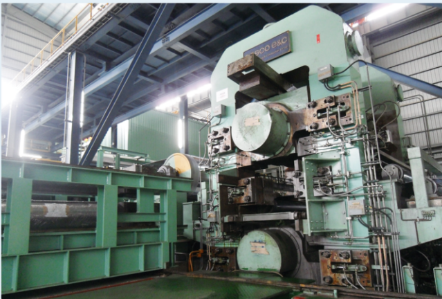
▲ 高張力整平、調質設備 Excellent tension, skin pass mill flatness facility
