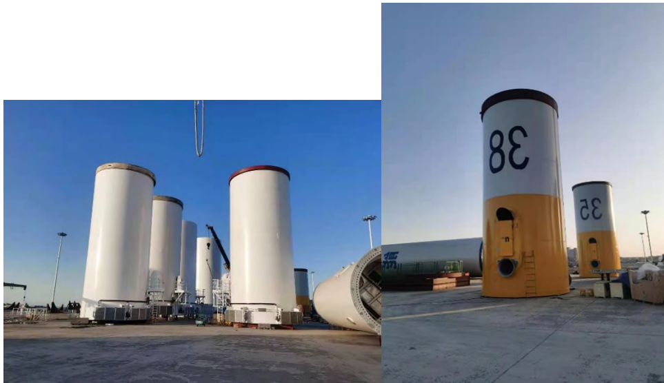
Some photos for offshore towers-bottom sections
