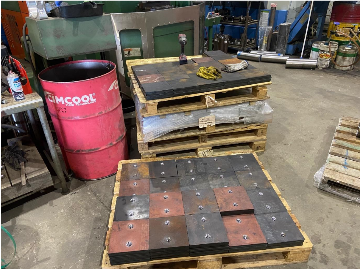
Mix of Bis450 and Chinese 450 Wear plate to be drilled and countersunk
