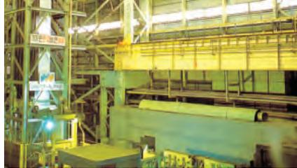
The scales from an HR coil can be removed completely by passing through the shot blast and pickling tank.
