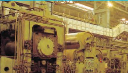
In order to obtain the flat shape and elegant surface, PosMAC3.0 product get passed through a skin pass mill. Also to prevent any white rust, product surface is coated with Cr-free or chromate to improve corrosion resistance property.
