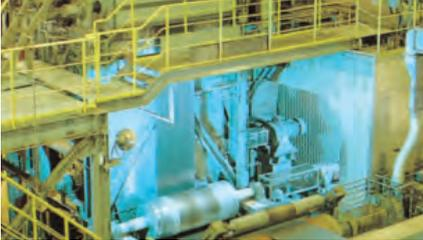
The equipments at the entry section are composed of two pay off reels and a welder.
