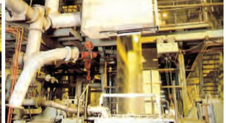
Zn-Mg-Al is coated onto the surface of the steel sheet after passing the annealing furnace in the pot reserved for PosMAC3.0, and then the targeted coating weight is achieved by spraying high pressurized air from the air knife.
