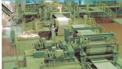
The equipment at the exit section are composed of an inspection table and an oiler equipment where the products are inspected synthetically and judged whether they are adequate for sale.
