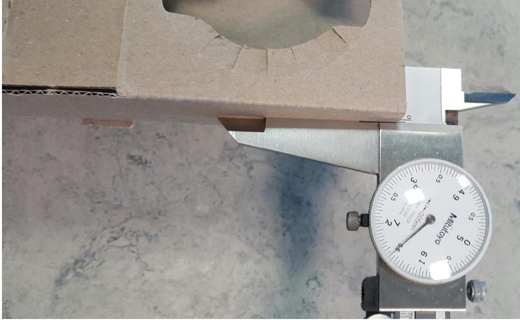
Figure 13 - thickness of McDonald's food tray, 1.5mm
