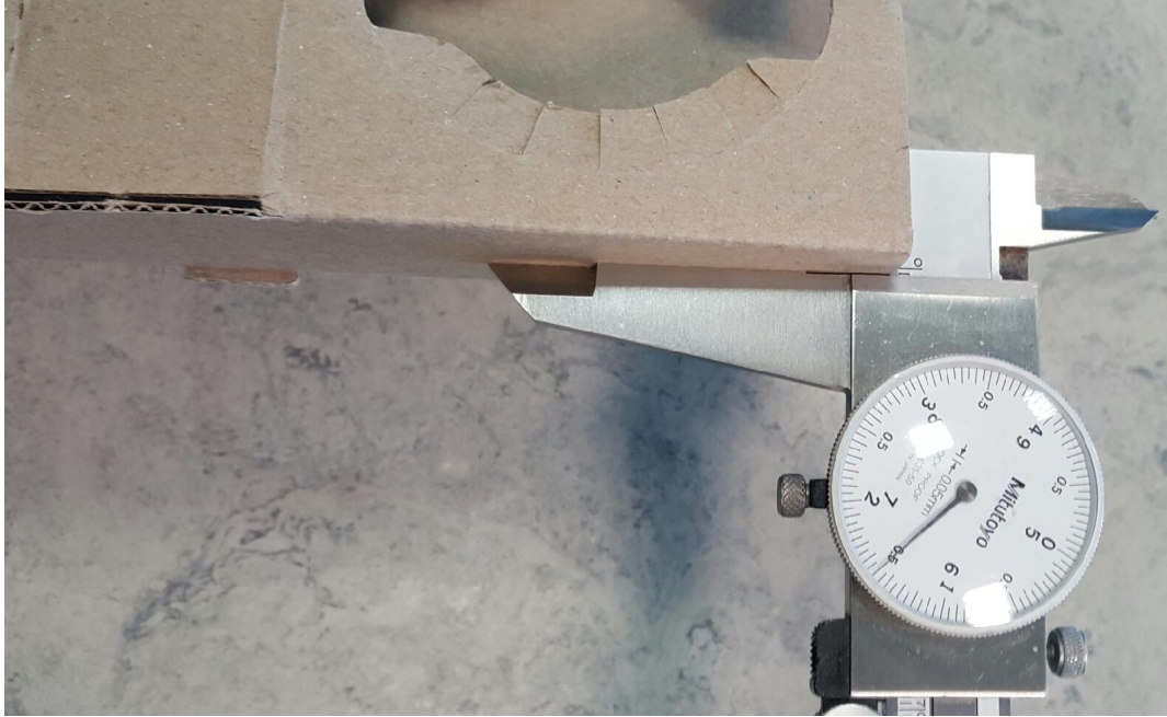
Figure 7 - thickness of McDonald's food tray, 1.5mm
