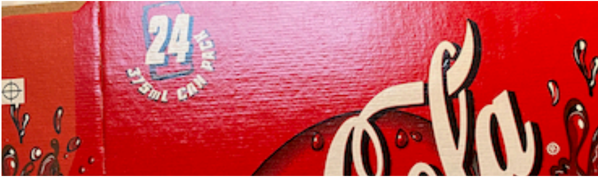
Figure 5 - Visy microflute showing "washboard" undulations
