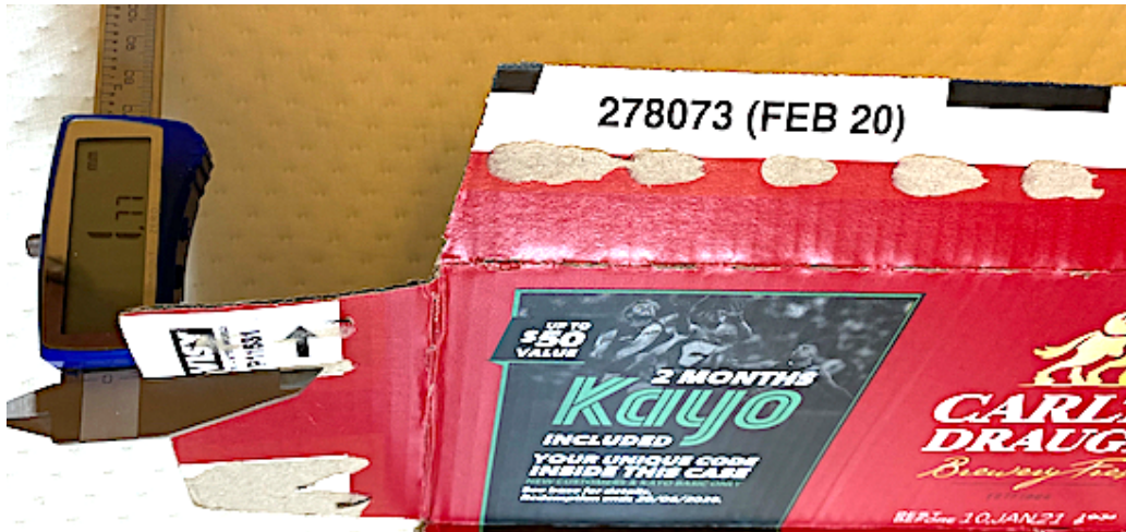
Figure 6 - Visy E flute beverage can multipack with thickness 1.77mm
