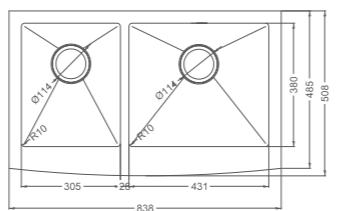
• High quality SUS304 stainless steel; • The content of chromium is above 18, and the content of nickel is more than 8.
