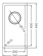
• High quality SUS304 stainless steel; • The content of chromium is above 18, and the content of nickel is more than 8.
