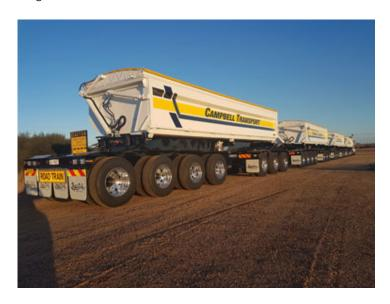
In 2006, BRE expanded its range to produce side-tipping trucks for the mining industry and have since engaged in lightweight body design using Hardox® 450 material grade— making them the lightest steel tippers in the market.
