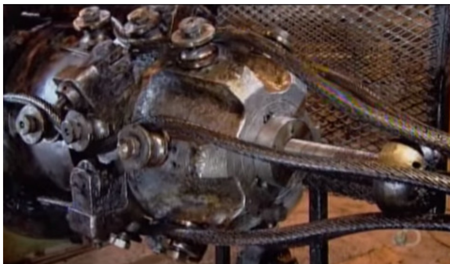
Figure 28: the six individual strands proceed from left to right, and are each pre-shaped by a series of rollers on the pre-former head.
