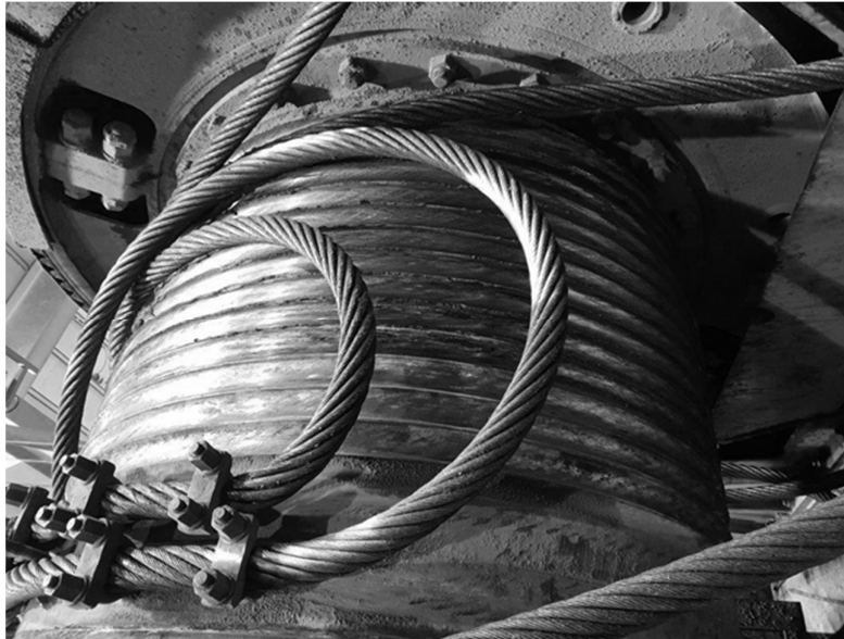
Figure 17: this is a photo of one of Scaw's 9 strand ropes bending quite significantly after an over-spool of the rope on the drum. The rope stayed intact and no deformation or kinking occurred. This rope was capable of being re-installed on the machine and saved the mine site six hours in downtime, plus the cost of another set of ropes.
