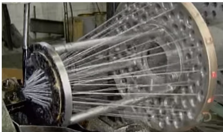
Figure 24: Aptly called a "strand forming point", the wires extending from the stranding machine converge and are wound together and covered in lubricant, forming a single, lubricated strand.
