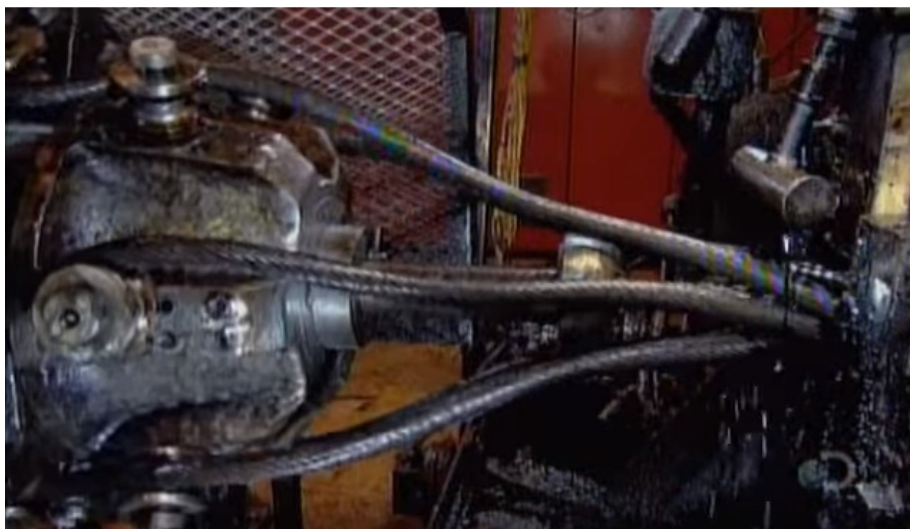
Figure 30: the rollers of the pre-former head pre-shape the strands into a spring-like form so they can be helically wound onto a core (right side of figure).
