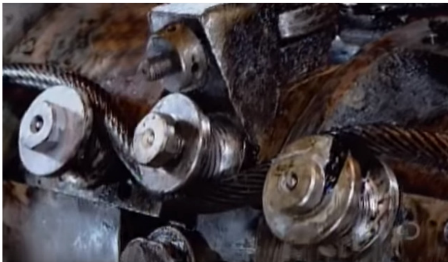
Figure 29: close-up of a strand being pre-shaped by rollers of the pre-former head.
