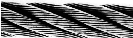
Figure 21: Right Hand Lay
