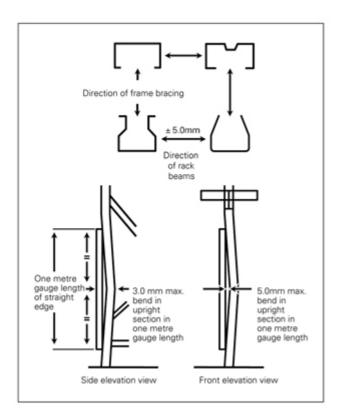
If an upright shows damage (see figure 4), is twisted or contains splits or cracks, replace it or splice in a new section. Splices should be approved by the racking manufacturer. Replace any damaged uprights and footplates.
