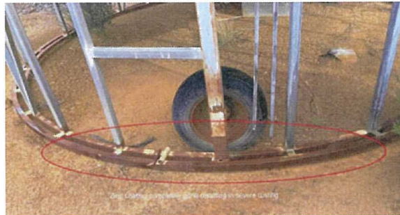
Picture 7. This picture is a close up of rusted Duragal® silo stand.
