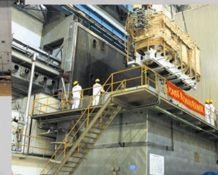
瑞士迈克菲尔公司煤油气相干燥装置 Vacuum drying equipment of kerosene oil-gas phase
