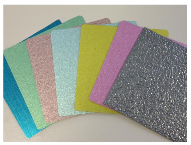
Tinted steel colours produced by Yieh Phui. The steel sample on the far right has a metal embossed finish.
