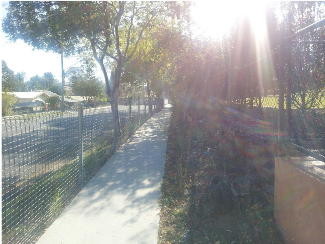
Photo 1 – Picture showing two fences. The fence to the right of picture has HDG air blown pipe as posts and the fence to the left of picture has pre-galvanised SHS posts
