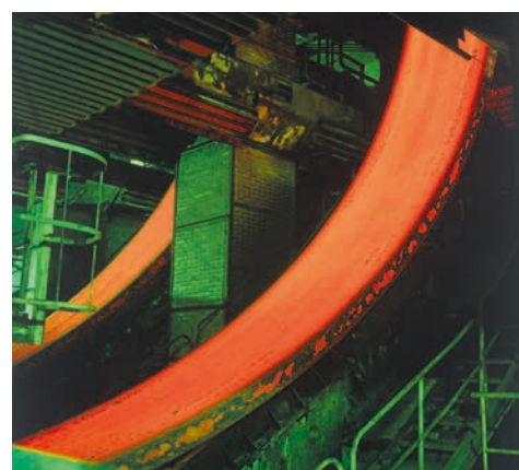
Continuous casting machine
