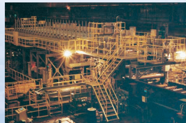
Super-OLAC (Online accelerated cooling equipment)
