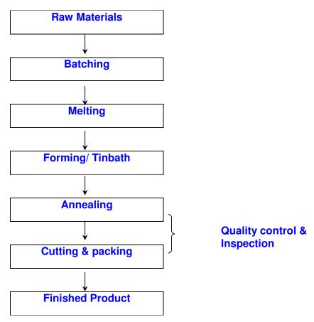
By-product in the form of cullets from the Cutting line are recycled wholly into production process as Raw Material.
