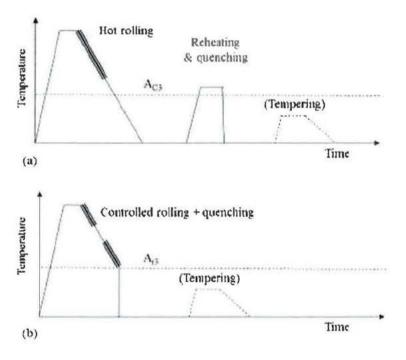
**Figure 1**. Temperature – time diagrams showing the differences between (a) the conventional production route and (b) direct quenching.
