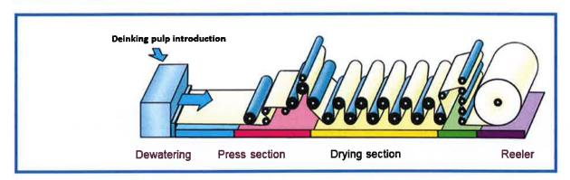
The newsprint manufacturing process involves the forming and drying of a thin web of pulp on the paper machine. Mechanical processes, such as pressing, and heating processes, such as drying, are used to remove water from the pulp as it progresses through the paper machine at approximately 1475 meters per minute. In case paper is rejected for quality reasons (before wrapping line) or damages (after the wrapping line), it is sent back to the repulping process. Trim loss is also repulped.
