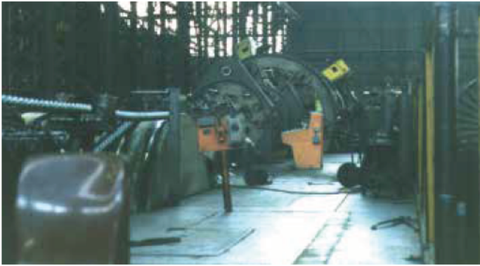
A length of rope being manufactured - usually in lengths of 1000m.
