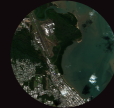
True colour composite appears as the human eye sees. This example is at 10 m spatial resolution from Sentinel 2.
