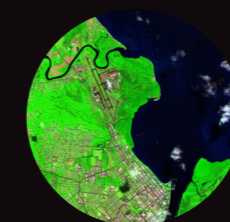
Short Wave Infrared (SWIR) showing plants in green, soil and urban structures in brown and water in black at 20 m spatial resolution. SWIR is also useful for showing newly burned land and mapping surface geology.
