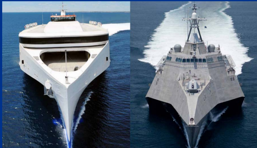
Figure 29: Austal Trimaran hull design used for both commercial and defence vessels
