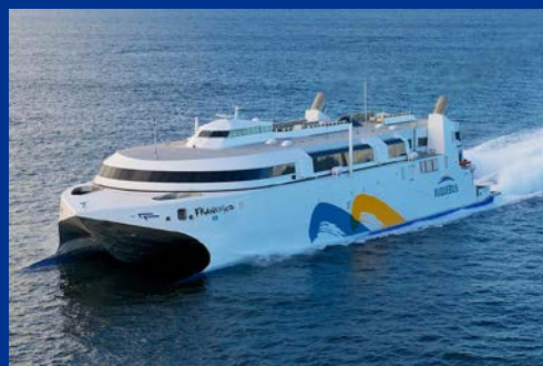
Figure 9: Francisco – the world's first LNG high-speed ferry, built by Incat
