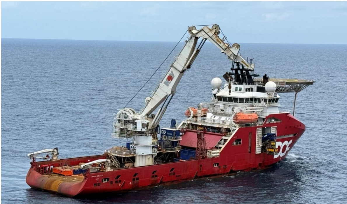
Figure 11: The Skandi Hercules launching a remote operated vehicle to cut the risers connecting the Northern Endeavour FPSO to the subsea infrastructure.
