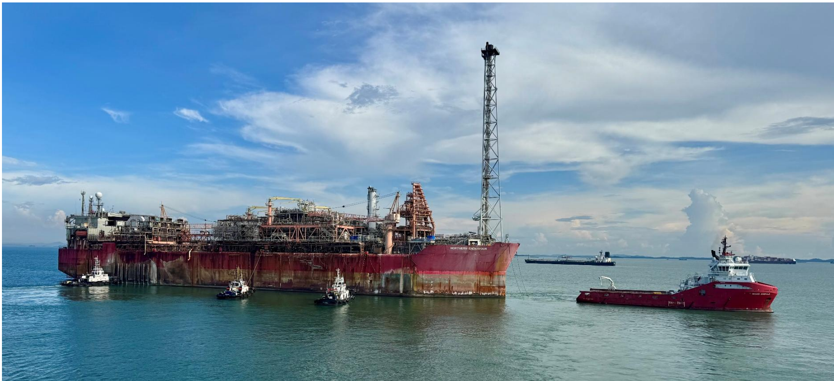
Figure 7: The Skandi Emerald and tugboats anchoring the Northern Endeavour FPSO at the mooring location in Singapore Harbour.
