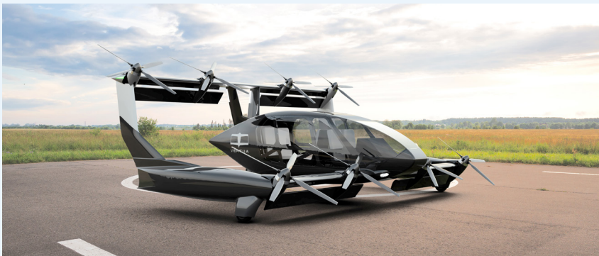
Australian designed Long-range hydrogen-electric vertical take-off and landing (eVTOL) aircraft.
