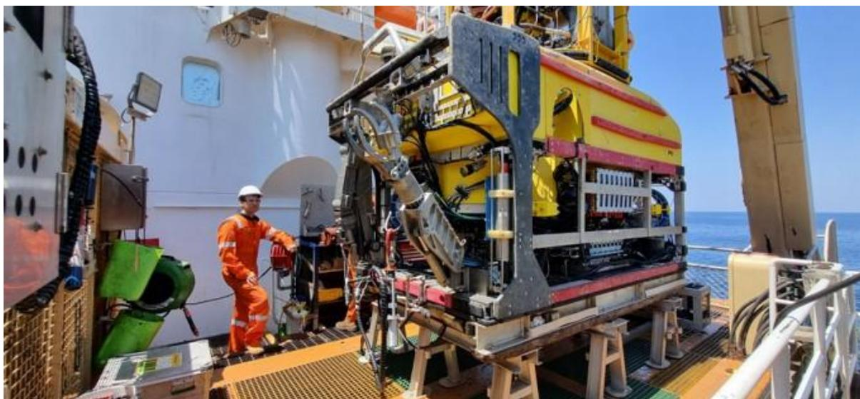
**Figure 5 – Remote operated vehicle on the Sapura Constructor preparing to do well suspensions.**
