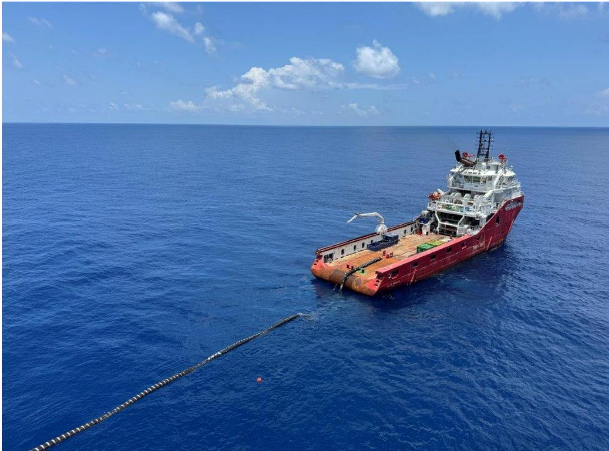
**Figure 3 – The floating offtake hose loaded onto the deck of the Skandi Emerald ready to be towed to Darwin for disposal.**
