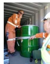
Figures 26, 27, 28 and 29 Drums of UOC being stowed into 20-foot ISO shipping containers.
