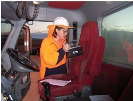
*Figure 8: Checking radiation levels in the truck driver's cabin.*
