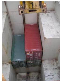
*Figure 9: Placement of containers into under-deck holds.*
