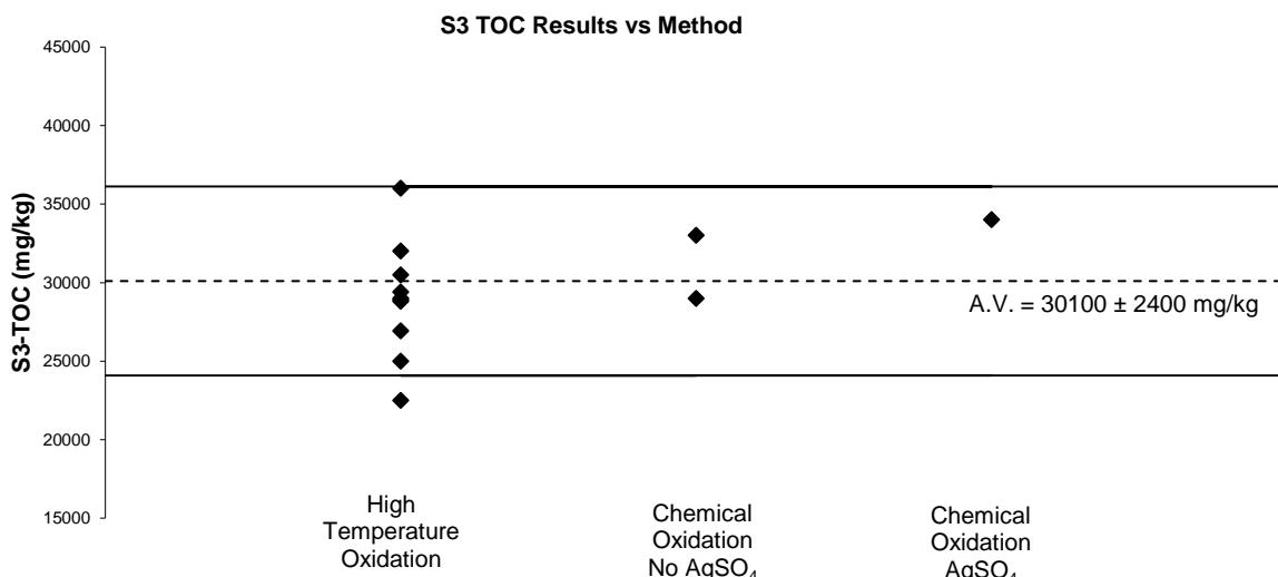
Laboratories 2 and 8 results of 2.9 mg/kg and 2.25 mg/kg have been plotted as 29000 and 22500 mg/kg respectively.
