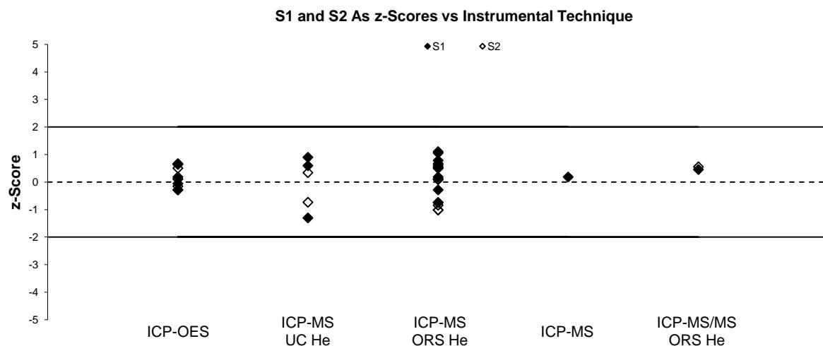
Figure 65 As Performance in S1 and S2 vs. Instrumental Technique
