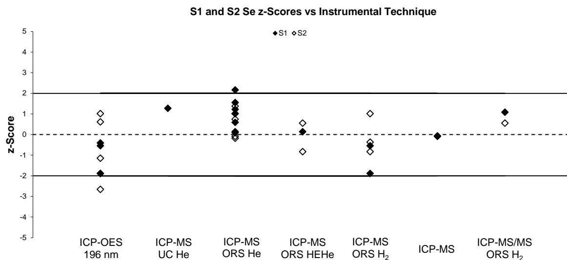
Figure 67 S1-Se and S2-Se Results vs. Instrumental Technique
