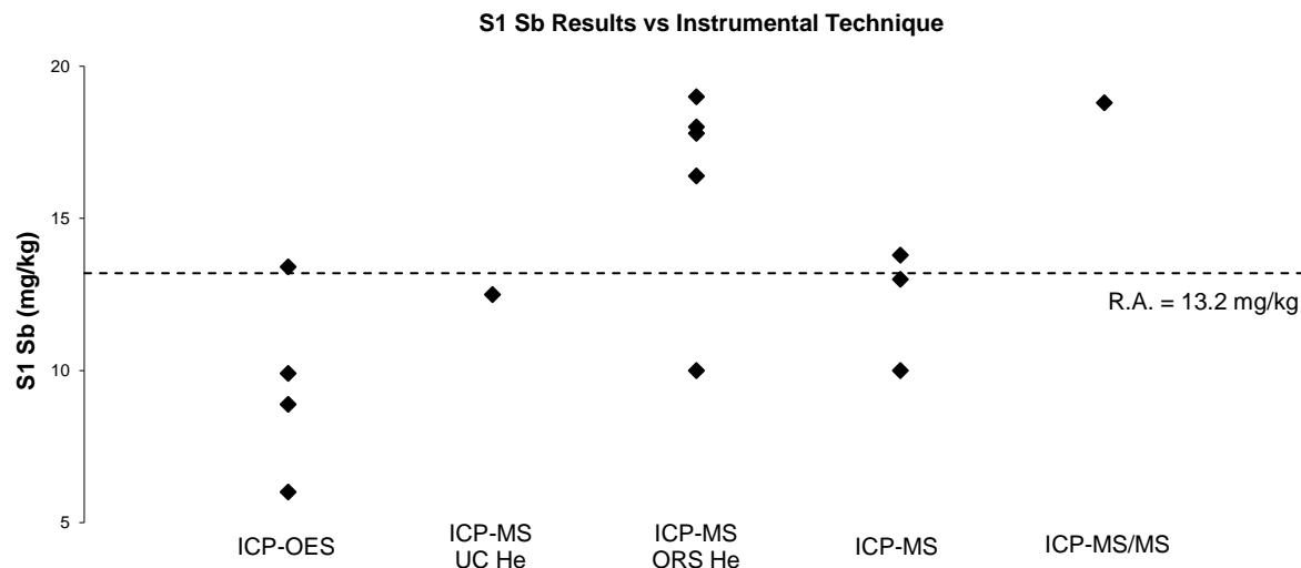
Figure 64 Sb Performance in S1 vs. Instrumental Technique
