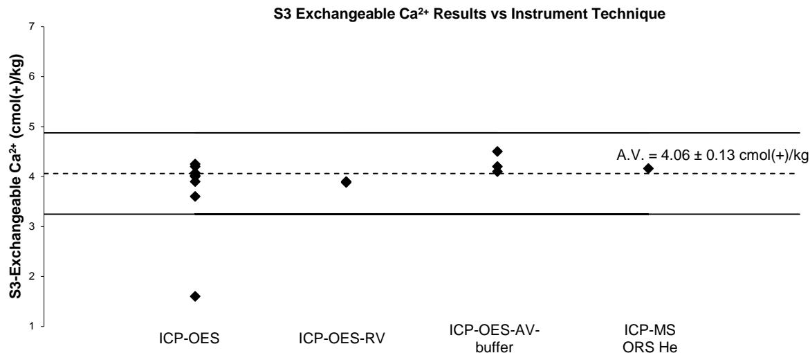
Figure 76 Exchangeable Ca<sup>2+</sup> Results vs. Analytical Methods
