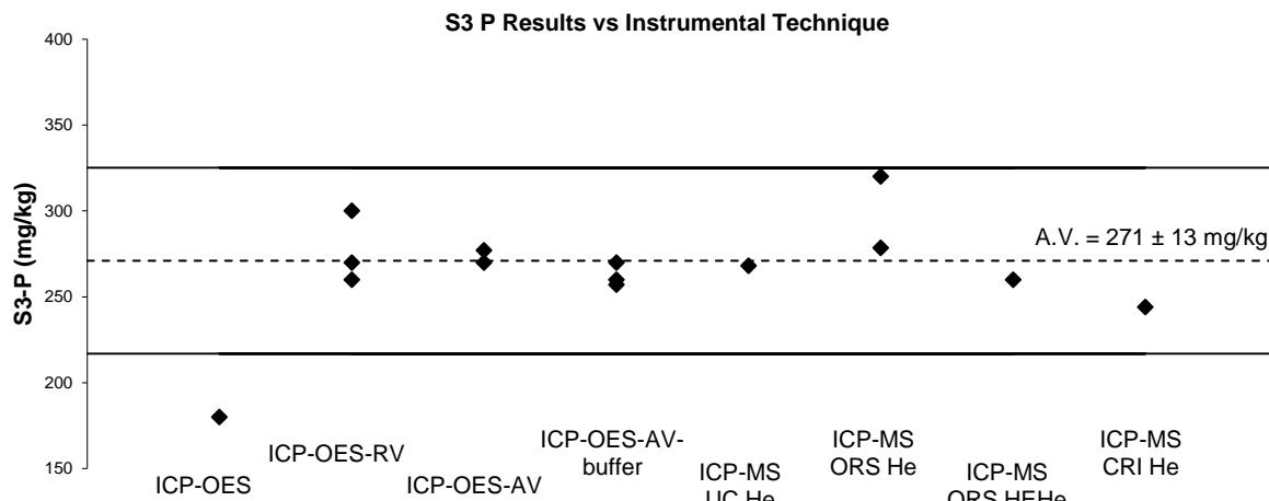
Figure 74 P Results vs. Instrumental Technique
