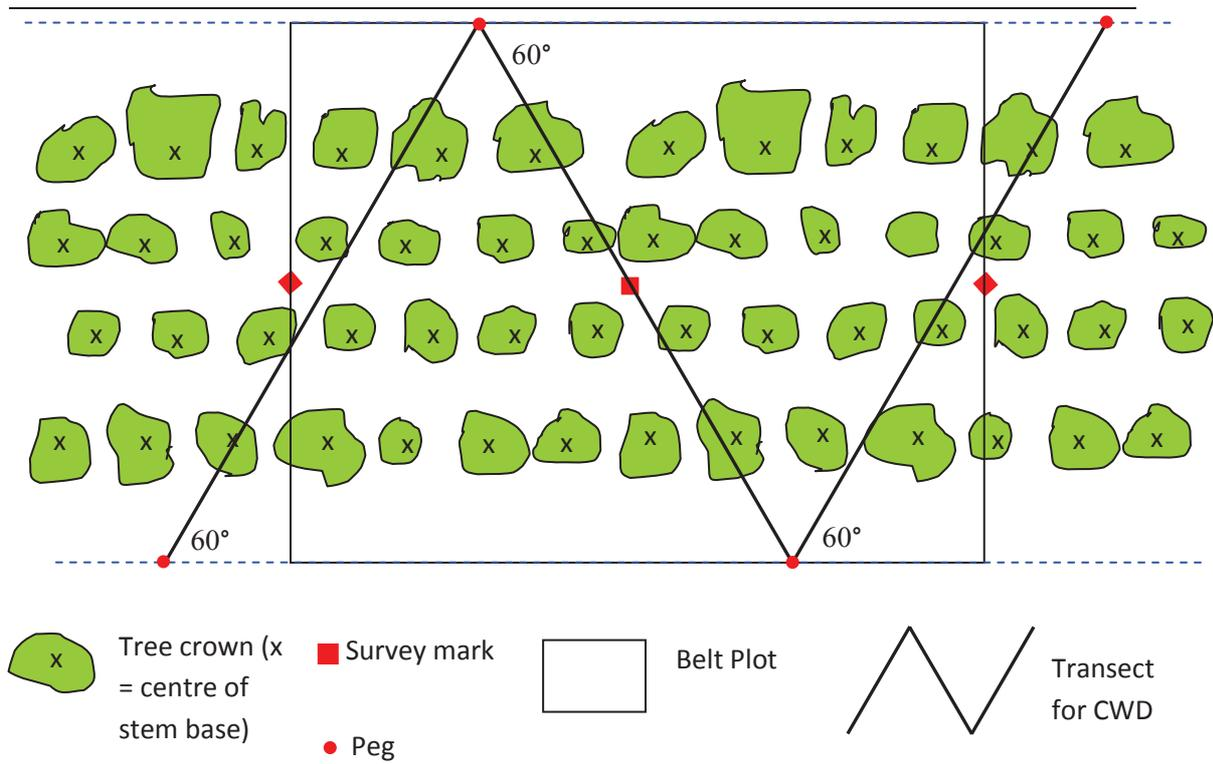
(2) Figure 11. Example of a 60° zigzag transect for CWD and litter estimation.
