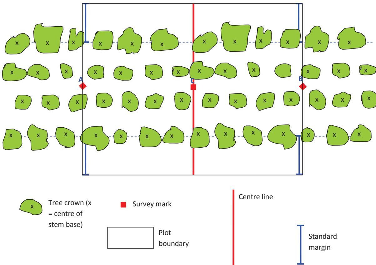
(7) Figure 4. Example of a belt plot in a belt planting with four rows. Distance AC = Distance BC = half plot length. Plot length (AB) is calculated to give the required plot area.
