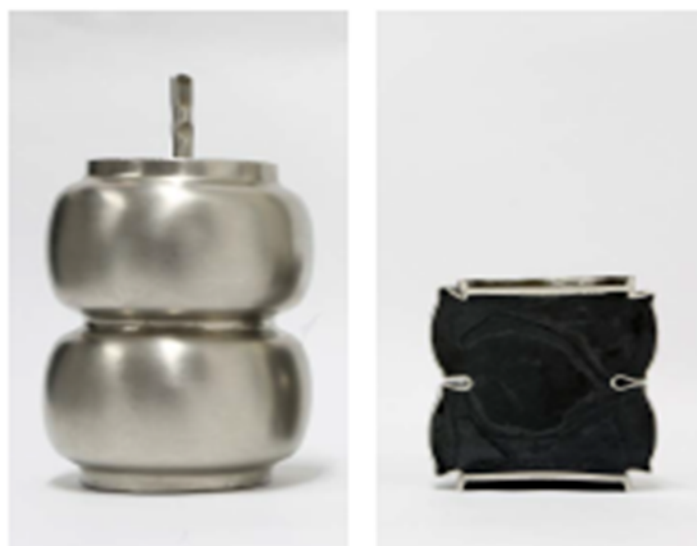
Figure 2: Waste in Synroc can pre-treatment and cutaway showing processed Synroc
