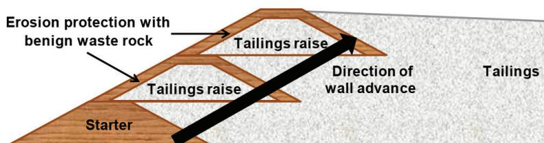
Figure 15: Downstream versus upstream raising
