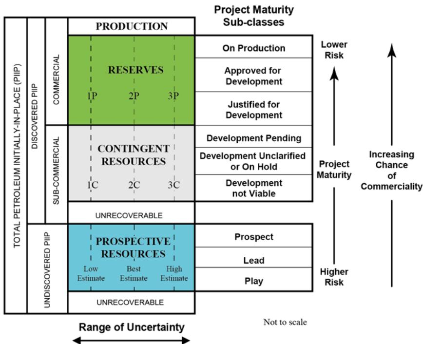
Figure 5. Hydrocarbon resource classification. The uncertainty range associated with hydrocarbon volumes decreases upwards, concurrent with the technical and commercial maturity of projects. Modified from SPE, AAPG, WPC, SPEE, SEG: Guidelines for Application of the Petroleum Resources Management System, November 2011.
