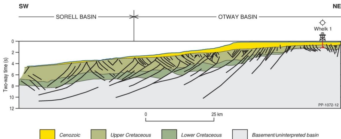
Figure A13: Cross-section of the Sorell Sub-basin which shows the transition from the Sorell Basin to the Otway Basin. Exploration targets in the Sorell Basin include the Shipwreck and Sherbrook supersequences (Upper Cretaceous) and the Wangerrip Supersequence (Cenozoic). Location is shown in Figure A12.
