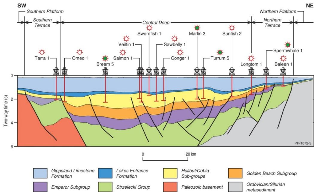
Figure A3: Cross-section through the central parts of the Gippsland Basin. Key exploration targets are present in the Latrobe Group, particularly the Cobia and Halibut subgroups. Location is shown on Figure A2 above.
